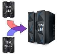
You can upgrade from any air-cooled zEC12 and z13 model to any z14 model. Upgrading from a water-cooled model is only possible to a z14 water-cooled model.
