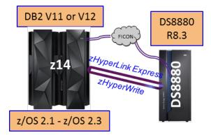
zHyperLink is a short distance mainframe attach link designed for up to 10x lower latency than High Performance FICON. zHyperLink will initially speed DB2 for z/OS transaction processing and later improve DB2 active Log throughput and VSAM applications.
