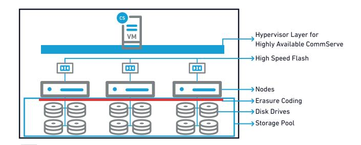
High Speed Flash – Used for Operating System, Commvault Binaries and Internal Databases.
